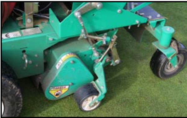
The working depth is determined by using the Height Adjustment Pivot Bar, the blades working down to a maximum of 40mm. Sand Injection with the Graden is designed to compliment hollow coring and not replace it.
