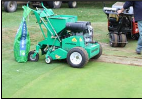
The Graden sand hopper holds 75kg of kiln dried sand. A typical golf green will consume between one to two tonnes per treatment depending on depth, a good team perhaps completing a green in under an hour.
