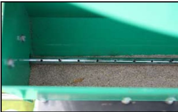
The Seeder Attachment is designed to cope with small grass seeds, including bent varieties. To get the best establishment, soil temperatures of 100 plus typically promote strong germination and seedling growth.
