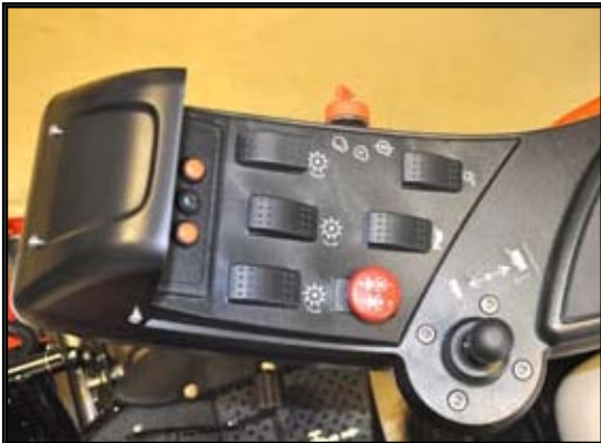
The armrest control on the all-electric Eclipse 322 will look familiar to existing Jacobsen greens mower users. The steering is also electrically assisted, the mower having no hydraulics on it at all.
