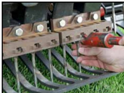
The Toro QuickChange system was introduced in 2010 and is a retrofit option for existing ProCore 648 pedestrian and mounted 864 and 1298 models.
