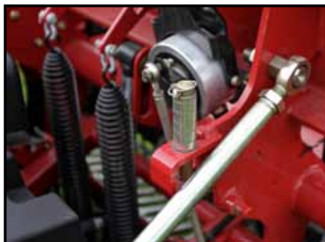
Adding or removing shims can control lateral float. The head can be fixed when aerating level surfaces such as a bowling green.
