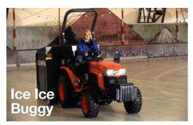
Staff at the Eden Project in Cornwall, have been using a Kubota B2230 compact tractor to power an Olympia 250 ice machine used to clean and prepare the ice for skate sessions.
