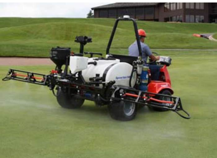
Spray Star sprayers from Ransomes Jacobsen are purpose built self-propelled units. Where a demount sprayer combination will be used full-time as a sprayer, it may be worth looking at a dedicated unit as an alternative.
