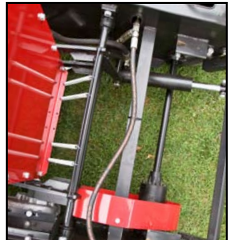
Simple driveline is designed to cut maintenance demands, the short drive chain requiring periodic lubrication. Note single hydraulic ram. This is used to raise and lower both the collection head and rear windrow swage boards.
