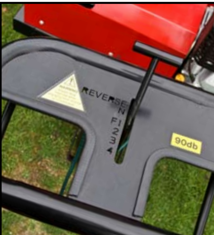
To engage drive, the operator pushes the control handle down; releasing pressure automatically brakes and holds the machine with no need to apply a park lock. Four forward ratios allow slow working to a brisk transport speed. In most conditions, the collector will keep pace with a pedestrian corer.
