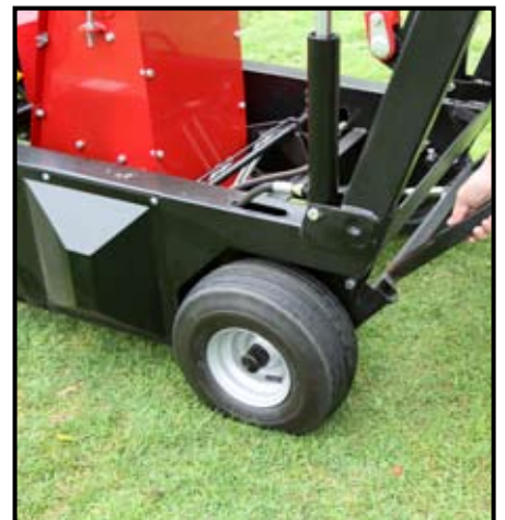
The swage board arms locate via a quick release system to allow them to be easily removed. When not in use, they can be stored in the hopper. This is useful when trying to cram a lot of equipment into a confined storage area. Note chain between the boards. This is used to set their working angle.
