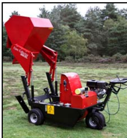
The 65kg / 1m 3 capacity hopper is designed to move forward as it tips for emptying, allowing it to fill a turf vehicle or low sided trailer. Lift height is put at 1.30m. Note tricycle design which is designed to allow good manoeuvrability.
