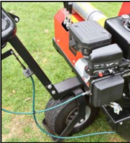
The original Charterhouse Core Collector CC3000 was powered by a 5.5hp petrol engine that featured hydrostatic drive. Introduced in 2006, the current CC3001HL model has a 7.5 hp Briggs and Stratton Vanguard power unit. See text.
