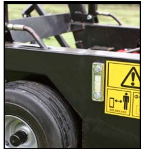
The main chassis rail on the left houses the 22 litre capacity hydraulic tank with its integral filter and sight glass level. The right chassis rail covers the pair of V-belts that take power to the rear axle drive chain; this drives the axle via a differential to prevent tyre scuff when turning.
