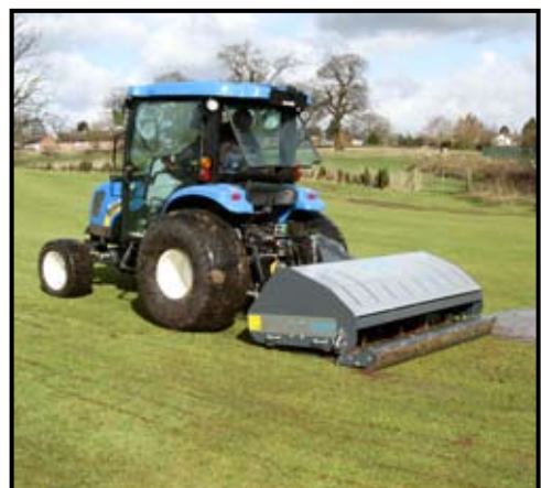
A collapsed drain provided a handy pool of water. Running the Shockwave through the waterlogged area speedily drained the surface water away.
