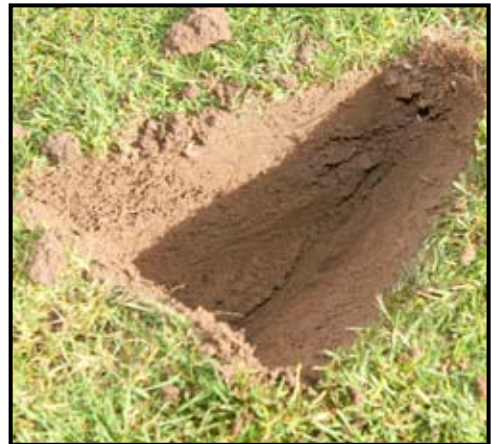
It is difficult to see in the photograph, but the test hole dug through a Shockwave slice can show how the turf has shuffled laterally across the working width of the machine.
