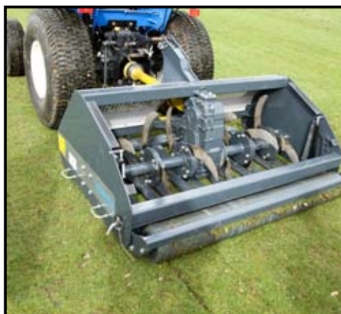
With its protective cover removed, the central gearbox and rotor shaft and blades can be easily seen. The forged blades wear in a manner that is designed to preserve the working depth; new blades have squared off ends.
