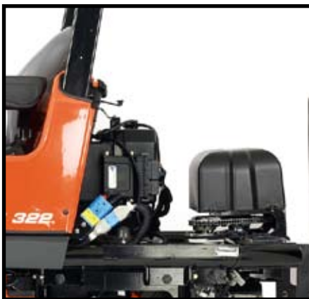
There is not a great deal to see under the engine cover, with good service access. Steering system is genuine 'fly by wire' and claimed to offer good 'feel'.
