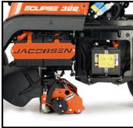
Nestling under the mower are extra batteries. These provide buffer energy to ensure instant power is always available to the mower.
