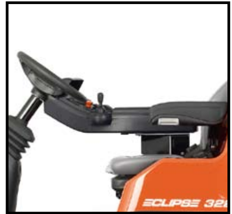
Jacobsen Command Arm and steering column are both adjustable. To sit on, the Eclipse 322 feels much the same as a Jacobsen diesel hydraulic mower.
