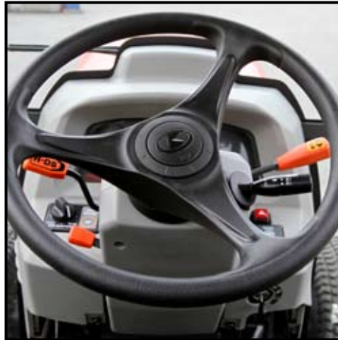
The steering column is home to the throttle (right), H-DS control (upper left) and (below left) the Auto Throttle Advance. The latter enables the HST travel pedal to also control the throttle, matching engine speed to the tractor speed in transport.
