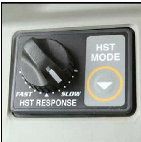
The HST transmission response is adjusted via a rotary knob (left), a push-button key (right) switching between transmission modes. Setting the tractor up to exploit various modes is not difficult. The transmission can be worked just like a conventional hydro using just the throttle and travel pedal.
