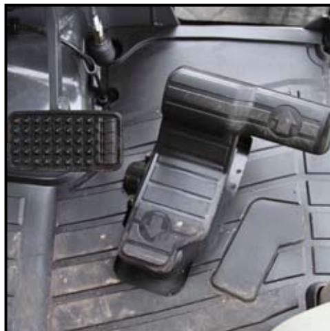
The servo-controlled travel pedal allows the operator to override the Cruise Control setting when making a turn or to alter the forward speed to meet a change in terrain or conditions. Once the pedal is released, the transmission will revert back to the cruise settings.
