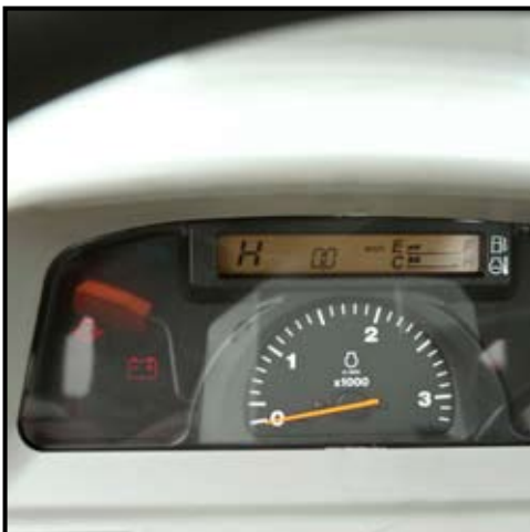
Where Kubota's HST Plus hydrostatic cruise control differs from normal hydrostatic drive is its ability to monitor and fix the forward speed using the tractors intellipanel. The digital display above the tachometer shows selected ratio on the left, a hare or tortoise symbol in green showing the selected high low split.
