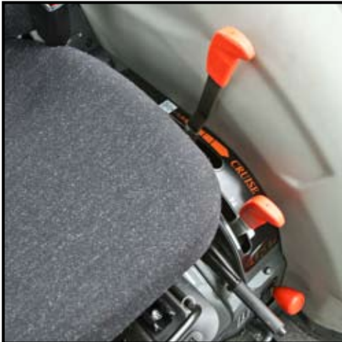
The Cruise Control lever is positioned next to the low, medium and high range selector. Once the desired engine speed and working ratio have been chosen, the lever is progressively eased forward to increase and then fix the forward speed.
