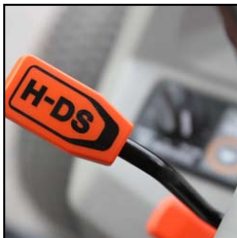
Hydro Dual Speed, H-DS, is operated via a steering column mounted lever. H-DS essential adds a high - low split which can be selected on the move. A typical use would be when using a loader, selecting 'low' for digging and 'high' when shuttling back and forth.
