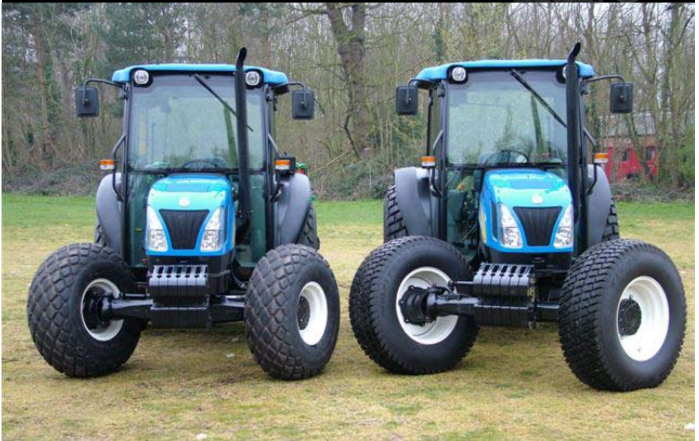
SuperSteer on the right has a pronounced effect on the agility of the tractor but the front tyres retain relatively flat contact with the ground, even at full lock.
