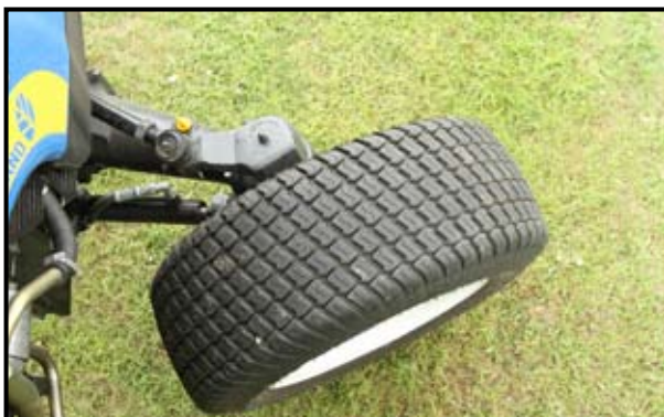
Viewed at full lock from above, note how the front wheel remains 'flat' at full lock. This is claimed by New Holland to help SuperSteer deliver a clean turn on fine turf.
