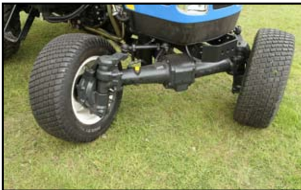
Pictured on a lower powered Boomer compact tractor, SuperSteer is now a widely available feature on New Holland tractors. Note axle movement across the front of the tractor.
