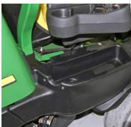
Below the command arm is a small cubby which can have a net cover. Greens mowers are designed to be light and compact, but a bit of storage space never goes amiss. Users can choose between smooth and tread pattern tyres.
