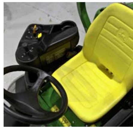
From the operator's point of view, there is little to tell the 2500B and 2500E apart from the seat. The latter mounted on a sloping rail to raise it as it is adjusted back. Steering column adjusts for reach.
