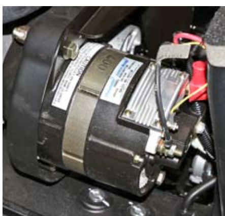
At a modest 2,250 engine rpm, the powerful alternator on the 2500E will deliver enough 'juice' to power the cutting units at the desired cutting speed. In work, the engine can be throttle back, cutting noise and fuel consumption.
