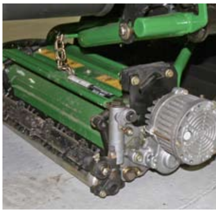
Brushless reel motors are well proven and liked for their ability to deliver precise cut speeds. As with all greens mowers, Deere places great emphasis upon quality of cut. Note the roller brush; users can specify a range of cutting unit options.
