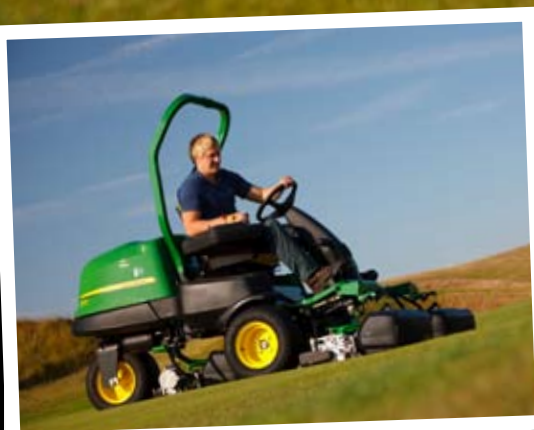
ABOVE AND LEFT: John Deere 2500 greens mowers come in two variants, the 'conventional' all-hydraulic 2500B and 'hybrid' 2500E. This uses a 48 volt alternator to drive brushless electric motors to power the units. The wheels use the same hydraulic system as 2500B.
