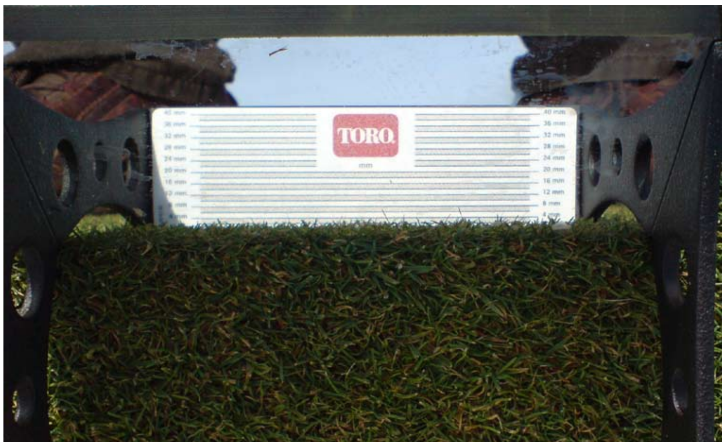
ABOVE: The TORO Turf Evaluator for measuring the effective height of cut
