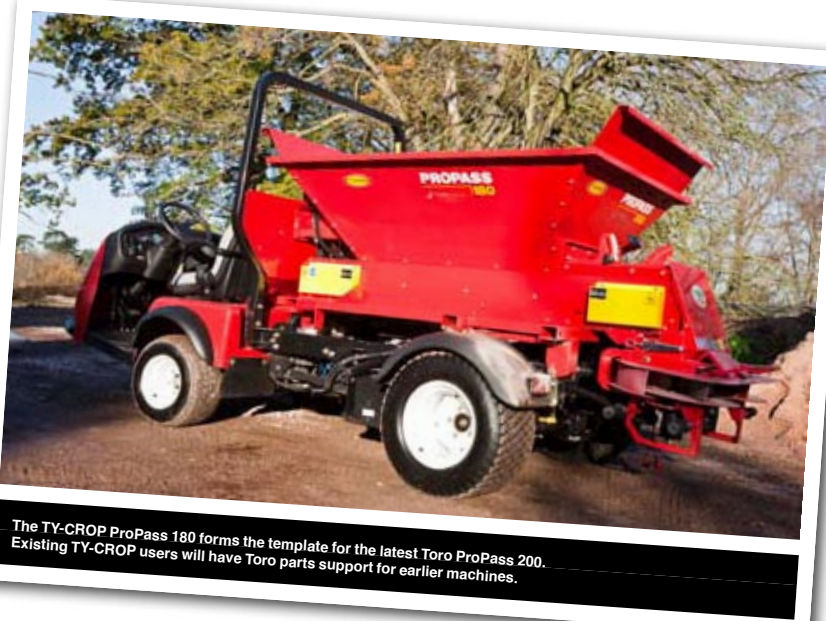
The hopper has smooth sides to help ensure the body empties fully. Existing ProPass users often fit a mesh grid over the hopper body to help break up any clumps as the unit is loaded.
