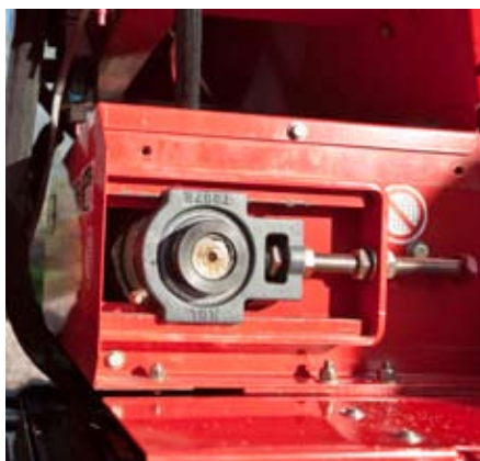
The hopper conveyor tension adjusters are easy to get at and are securely mounted. Note grease point and heavy-duty bearing. HSE regulations mean some of the lube points can only be accessed once a bolted on cover has been removed.
