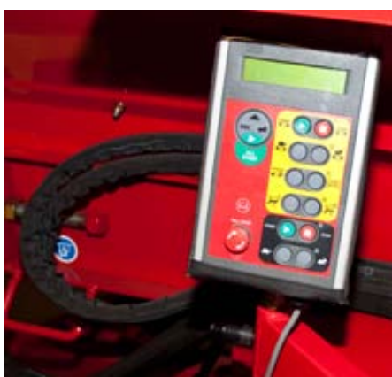
An electronic control box is standard, and makes setting the conveyor and spinner speeds straightforward. The Wireless Controller does the same job, but can be operated remotely.
