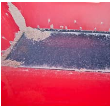
The hopper has smooth sides to help ensure the body empties fully. Existing ProPass users often fit a mesh grid over the hopper body to help break up any clumps as the unit is loaded.
