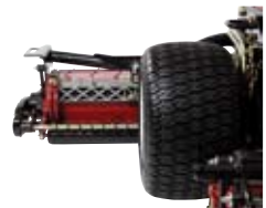
The cast alloy Toro DPA units are now well established, their fitting to the 3100 series extending the range of cutting units options available.
