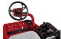
The Toro 3100 operator platform is simple and clutter free. Note the simple inclinometer.
