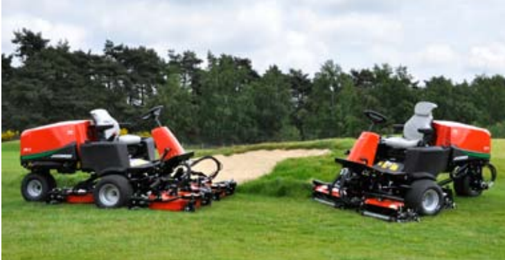
The Jacobsen rotary deck AR3 and cylinder TR3 utilise the same three-wheel hydrostatic three-wheel tractor unit.
