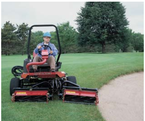
Where the Sidewinder option is specified, all three cutting units can be offset to work 610mm to the left or right. This allows mowing close to vulnerable bunker edges or to be used to alter wheelings around surrounds.
