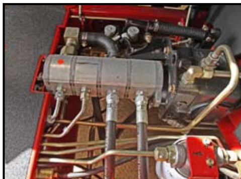
Separate pumps are fitted for steering, traction, unit raise and reel drive. Note extensive use of solid hydraulic lines. Behind the pumps are the valves that are used to set the reel speed in relation to forward speed. Consistent clip rate is claimed for an even finish.
