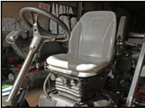
Operator orientated features include adjustable side arm and steering column. The seat can be specified with pneumatic suspension. This has the advantage of automatically setting the spring rate to suit the weight of the operator.
