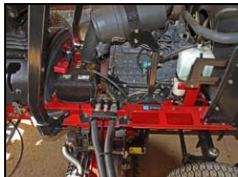
The rear engine hood tilts to provide good daily service access with all check points, including the battery, on the same side. Open frame design aids cooling and helps to prevent debris build-up around key components.
