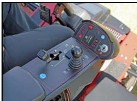
Adjustable side arm houses key controls. It can also be raised to allow access from the offside; useful in sheds where the mower may be parked with poor nearside access. Visibility from the seat and a general lack of clutter make it easier to accurately place the mower.
