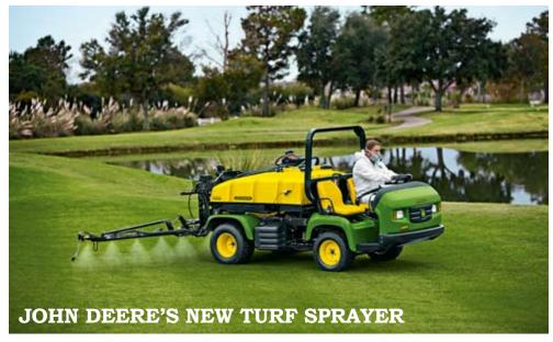
John Deere's new HD200 SelectSpray machine is an upgraded version of the 750-litre low profile sprayer first introduced in 2003.
