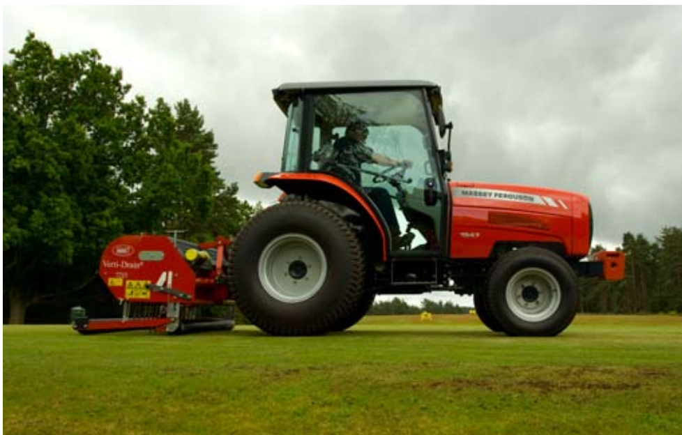
TOP: The bunkers at Hankley Common Golf Club are of a fair size and a couple used to suffer from puddling after a heavy night's rainfall. The solution was to run a pass through with the Verti Drain.
