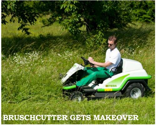
Etesia's new Attila SKF 85cm brushcutter has a totally different 'look' to previous machines in the Attila range. Designed for clearing the thickest of brambles. bracken, saplings and dense undergrowth, this latest ride-on cuts its way through virtually everything in its path, reducing overgrown vegetation to mulch.
