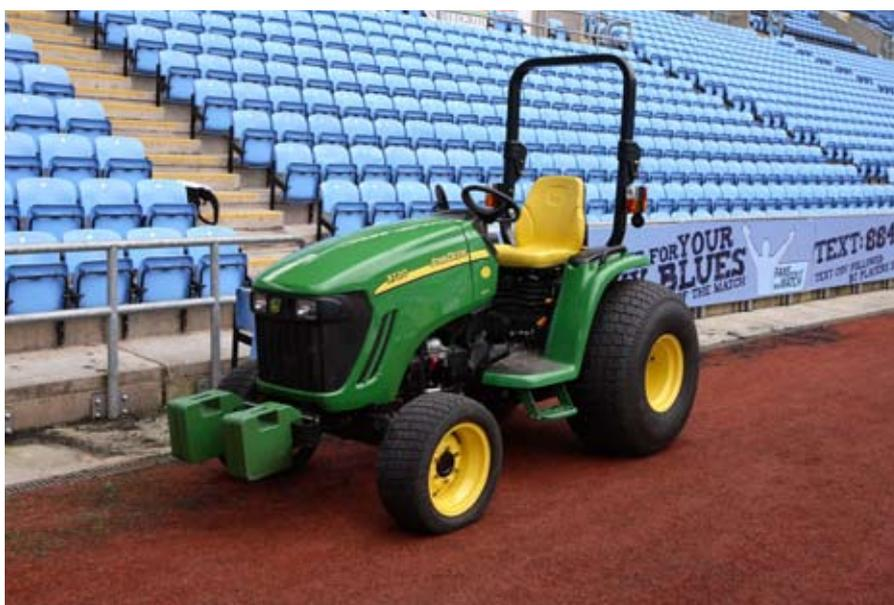
The eHydro transmission option on John Deere 3720 tractors offers all the features of a conventional hydrostatic drive with added control. It is easy to set up the tractor to run at a fixed forward speed, even after changing the throttle setting.
