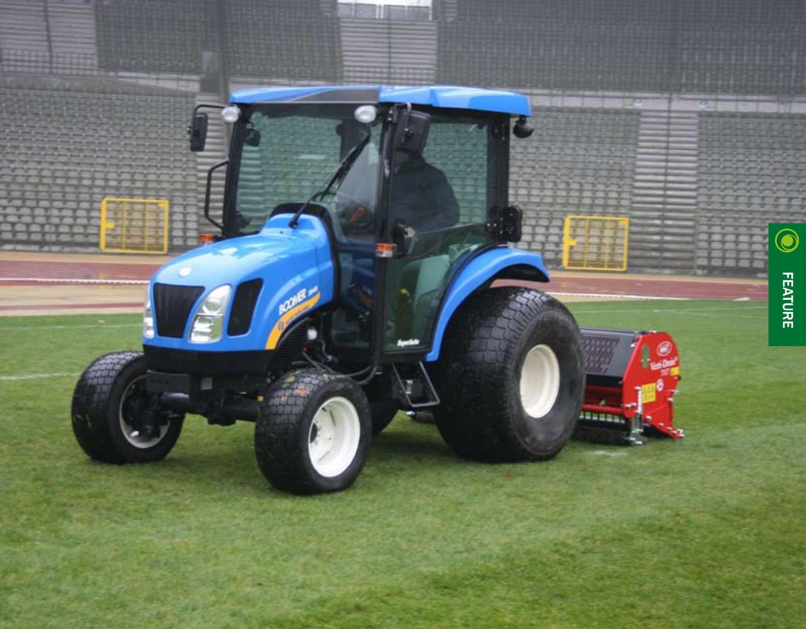
In applications, such as mowing, the New Holland EasyDrive can be operated just like a hydrostatic transmission tractor, the operator either using the floor mounted travel pedal to 'manually' vary the driving speed or fixing a 'cruise' speed that can automatically take into account varied load on the PTO.
