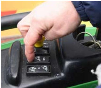
With the John Deere eHydro transmission, setting a fixed working speed is simple; use the travel pedals to attain the desired speed and press set. The speed can then be fine tuned, on the move, using the same switch.
