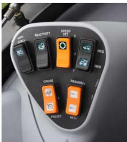
EasyDrive is set up using a set of buttons mounted to the left of the operator. The main buttons are pretty easy to understand, with only Speed Set needing a bit of understanding. This control is essentially used to cap the tractors speed to 30%, 60% or 100% of maximum, in effect changing the sensitivity of the travel pedal to suit different applications.
