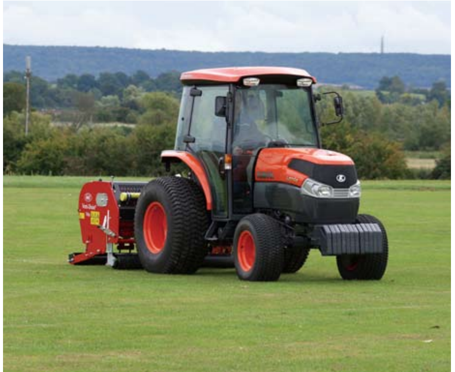
Kubota offer its HST Plus hydrostatic transmission on its GL40 series, advanced features enabling the operator to select fixed cruise and automatic engine idling features. The key is to look more deeply into what transmissions are on offer and not assume they are all the same.
