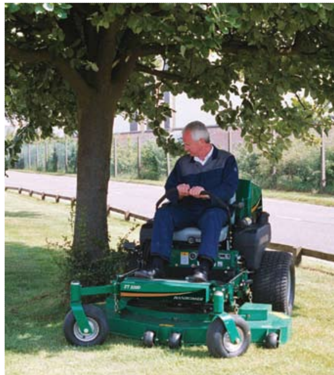
Powered by a 20hp Yanmar diesel, the Ransomes ZT220D has a 1.50m deck. Small and nippy, this mower is ideally suited to working in and around trees, flower borders and other obstacles.
