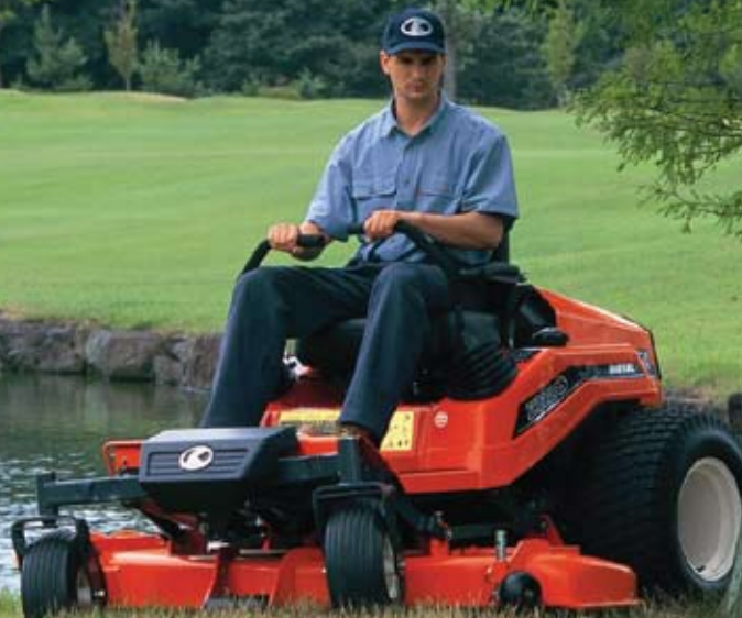
Kubota zero-turn mowers are all diesel powered, the pictured ZD28 topping the four-model line-up. Powered by a 28hp engine it can be specified with a choice of 1.52m side- or rear-discharge deck.
