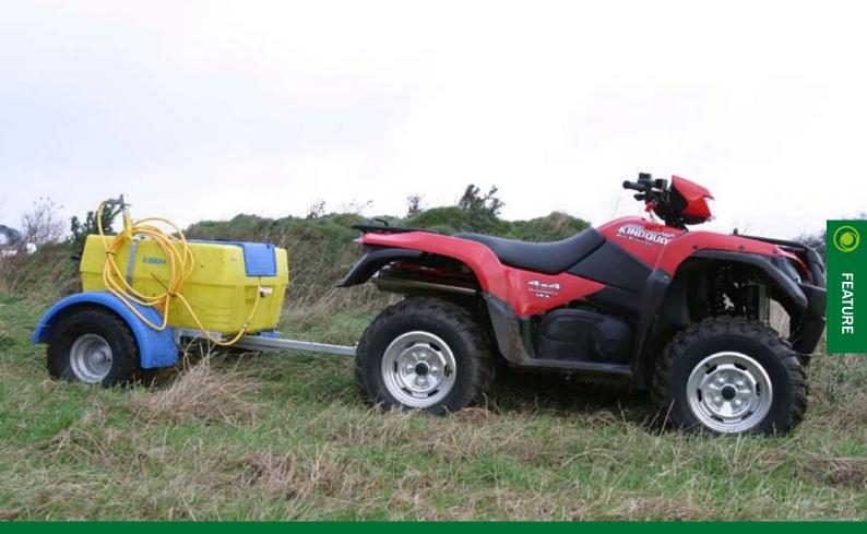
Trailed attachments have the added advantage of fitting behind both ATVs and utility vehicles. On level terrain a light, 2WD ATV will pull around 250kg, more powerful models coping with double that even over rougher terrain.
