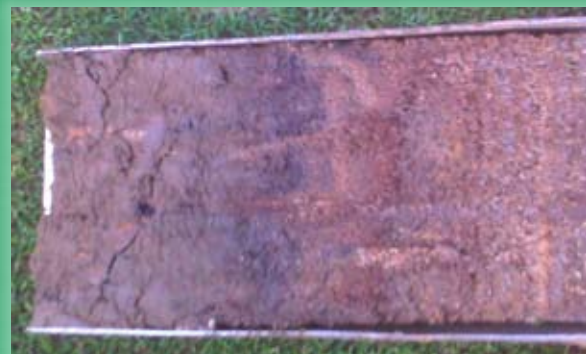
Dead soil of with excess thatch iron bands, black layer, compacted soil, no life and no roots.
