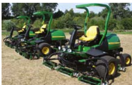
A turbocharged 36hp engine powers the 7000 Series, with a turbocharged and intercooled 42hp unit driving the 8500.
