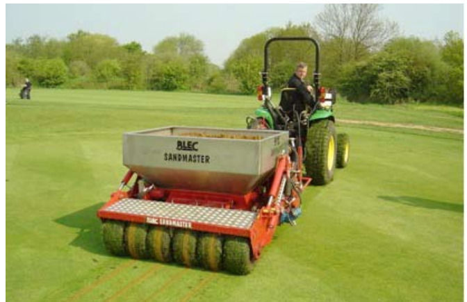
Rapid, one-pass installation of small sand slits at close
