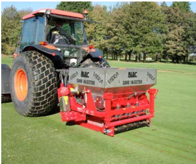
Neat one-pass slit installation by sand injection
