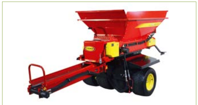
Distributed in the UK by Turfmeh Machinery, the TYCROP ProPass 180 ultra low impact broadcast top dresser can be used as a large-area top dresser fitted with twin rear spinning discs or, with these removed and the optional swivelling cross conveyor fitted, used as a bulk loader for filling trailers or greens top dressers, bunker filling, tee construction and path resurfacing. The conveyor measuring 203mm (8in) wide by 1.65m (65in) long and will through an arc of 180 degrees. All Tycrop models feature a simplified instructions to adjust application rates
