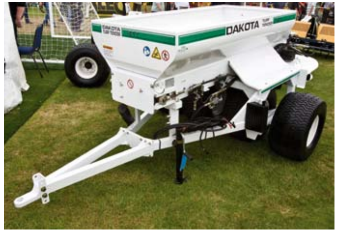
Campey Turfcare Systems established the Dakota 'Turf Tender' top dresser range in the UK, with mounted and trailed units spanning 0.65m 3 to 3.82 m 3 . Spinning disc models spread up to 10m, the Dakota set-up system making these machines popular with operators. As with all types, the choice of model will need to be related to the machine's intended applications and the equipment that will operate it.
