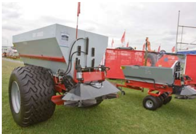
Taking a side by side look at Rink top dressers from Charterhouse Turf Machinery shows how the designs offer different approaches to wheel and tyre positioning. It can be wrong to assume a smaller and lighter machine will always have a lighter footprint. Mounted Rink models start at 1.0m 3 capacity and spread to 1.5m, the large 3.8m 3 DS3800 on the left offering spread widths from 2.0 to 15.0m. Material can be applied to a thickness of between 0.5 to 15mm.
