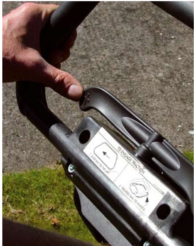
... the thumb operate lateral control having '+' and '-' to the left and right to increase or decrease mowing speed.
