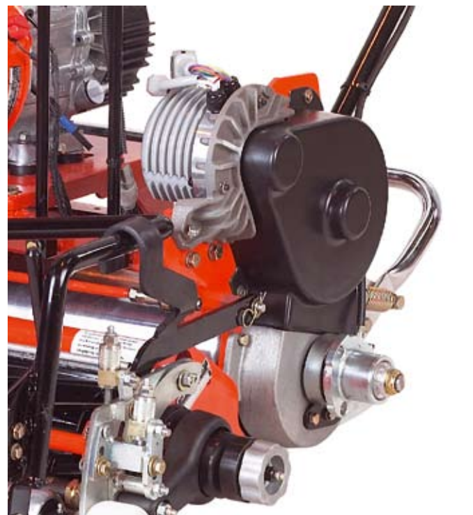
A second electric motor on the Eclipse 122 drives the rear roller. Its speed can be easily varied
