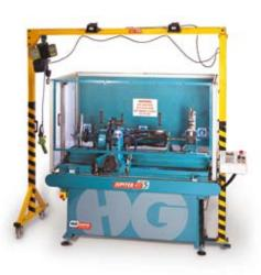
The new version 3 software identifies the various applications available for simple selection. including a dedicated programme for bed knife grinding with variable traverse speed. A new electronic braking facility also adds to the ease and accuracy of set up.
