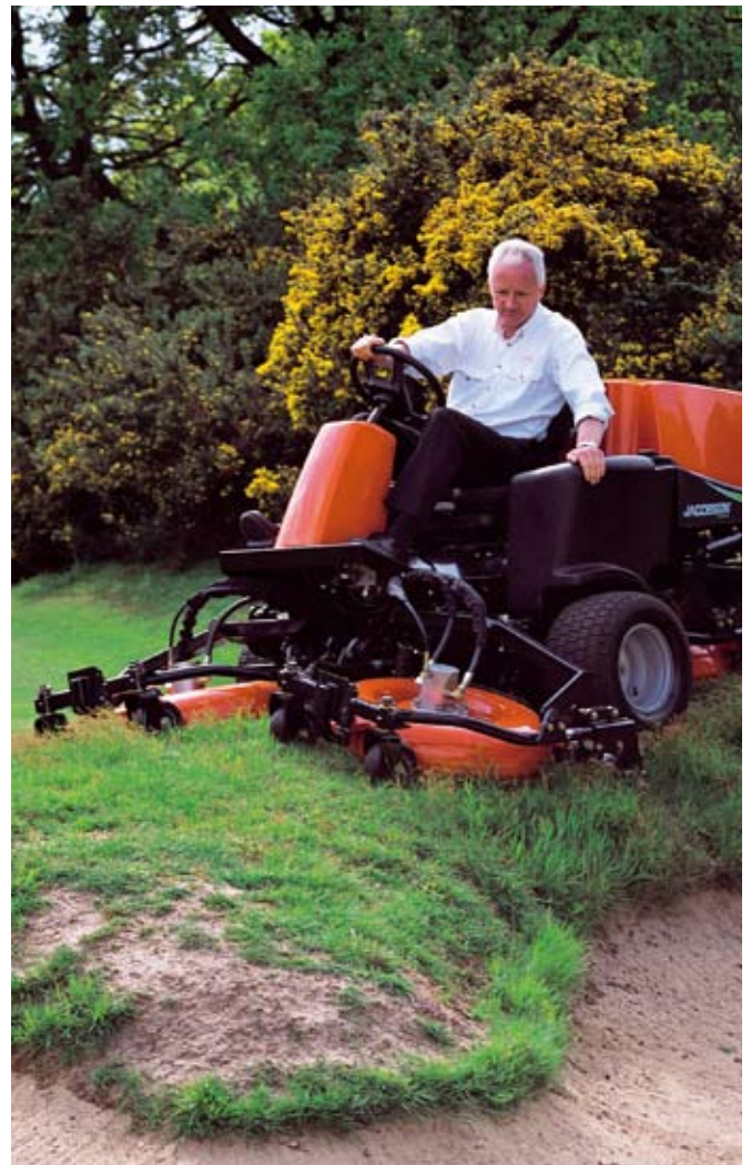
As demonstrated by this Jacobsen AR3, ride-on access to difficult to access areas is a key rotary mower strength. This particular model is purpose designed for this type of work, three-wheel drive and a pokey 33hp diesel combining traction and power
