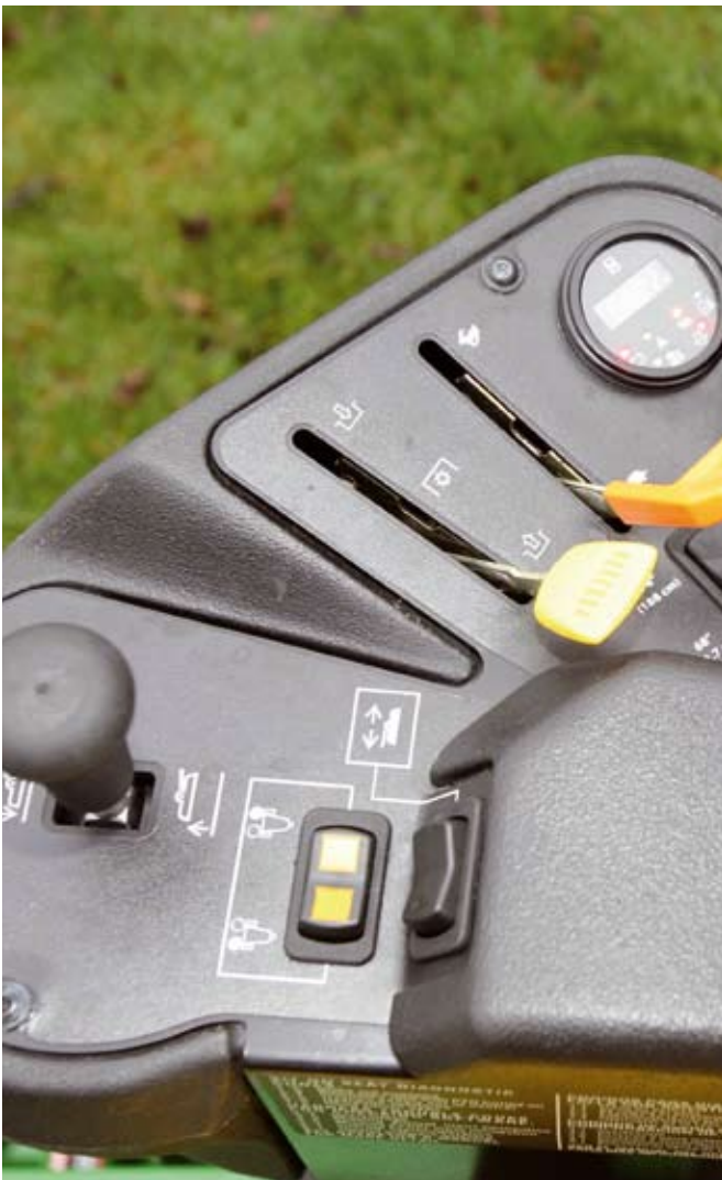
The controls on the John Deere 7400 are extremely simple. All it takes to adjust the mowing width or push out an outer unit is the touch of a button. The mower is a joy to use, with low noise and vibration levels
