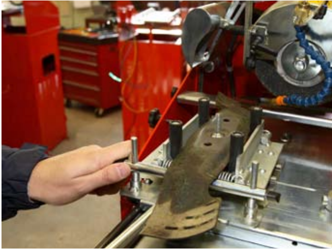
Rotamaster 4000 is able to accommodate most types of rotary blade, the machine's carriage incorporating a simple spring clamp with adjustable bar rest to keep it securely retained as it is sharpened.
