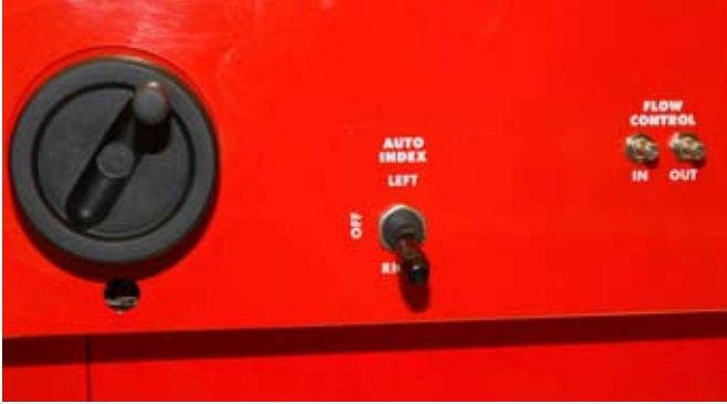
The carriage is set to the left for right-handed blades.
