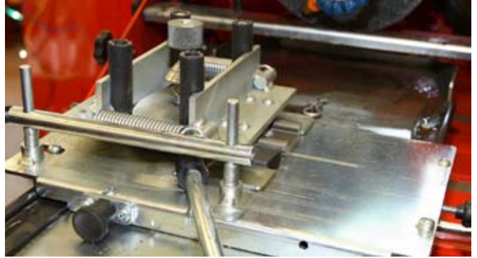
The carriage is set to the left for right-handed blades.
