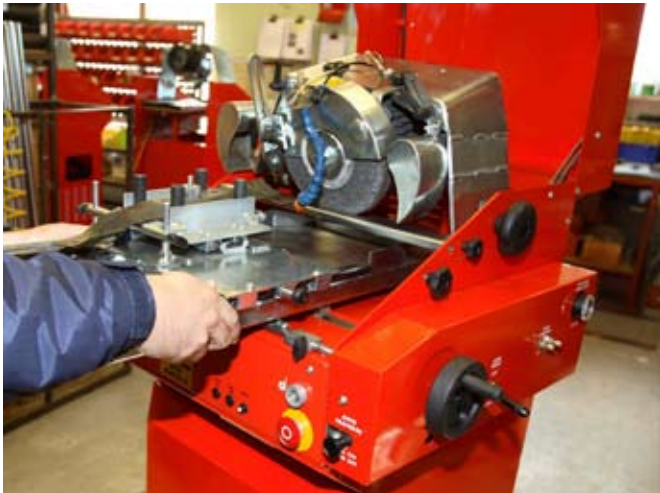
The distance the carriage travels across the face of the grind stone is set by setting manual stops. Once set for a specific blade type, this setting can be retained. Micro switches trigger the pneumatic ram powering the carriage to change direction.
