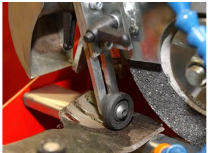
A simple jockey wheel can be lowered onto the blade so the grinding wheel follows a ramped profile. Simple and effective, it ensures consistent sharpening across the area to be ground.
