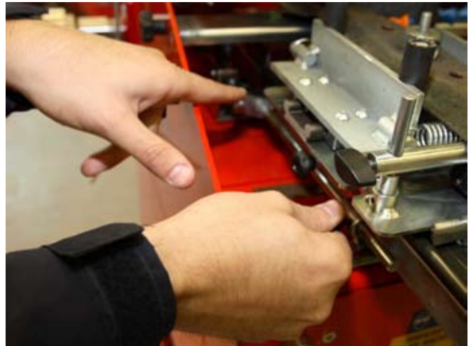
Doing a dummy run with the carriage pushed in and out by hand is recommended. This allows the amount of travel to be fine tuned to suit the blade. Note also the adjustment incorporated for the rear blade support.
