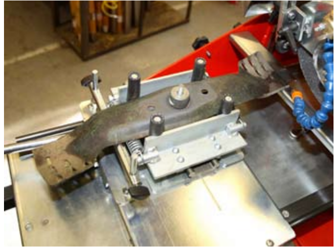
For added security, a quick thread nut secures the blade through its central bolt hole. Note how the tip of the blade rests on a cross member. This provides support as the carriage moves back and forth. Blade sharpened light end first.
