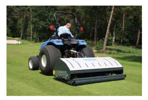
Now finished in silver-grey and black, the Imants range of de-compaction and slitting equipment from Campey Turf Care Systems is offered in a broad range of sizes to suit both in-house and contract operations. The pictured Shockwave 2.20m will relieve compaction down to 35cm, its drop forged rotary slicing times shuffling the soil laterally to relive compaction across the machines width. Also offered in 1.55 and 2.10m widths.
