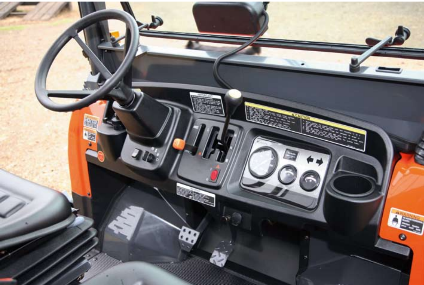
Kubota controls are well thought out and easy to understand, the quality of the fit and finish certainly having more in common with a road vehicle than most utilities. On-road pep not great but on off-road tyres this is no bad thing. Power steering is standard.
