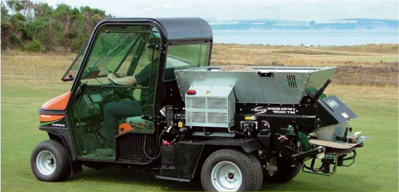
Kubota offers its well-proven RTV900 in road-homologated form. Fitted with a screen and ROPS frame, the unit has individual front seats with suspension for the driver, full road lighting and a front 'crash bar'. Full hypostatic drive means there will be little need to trouble the brake pedal.
