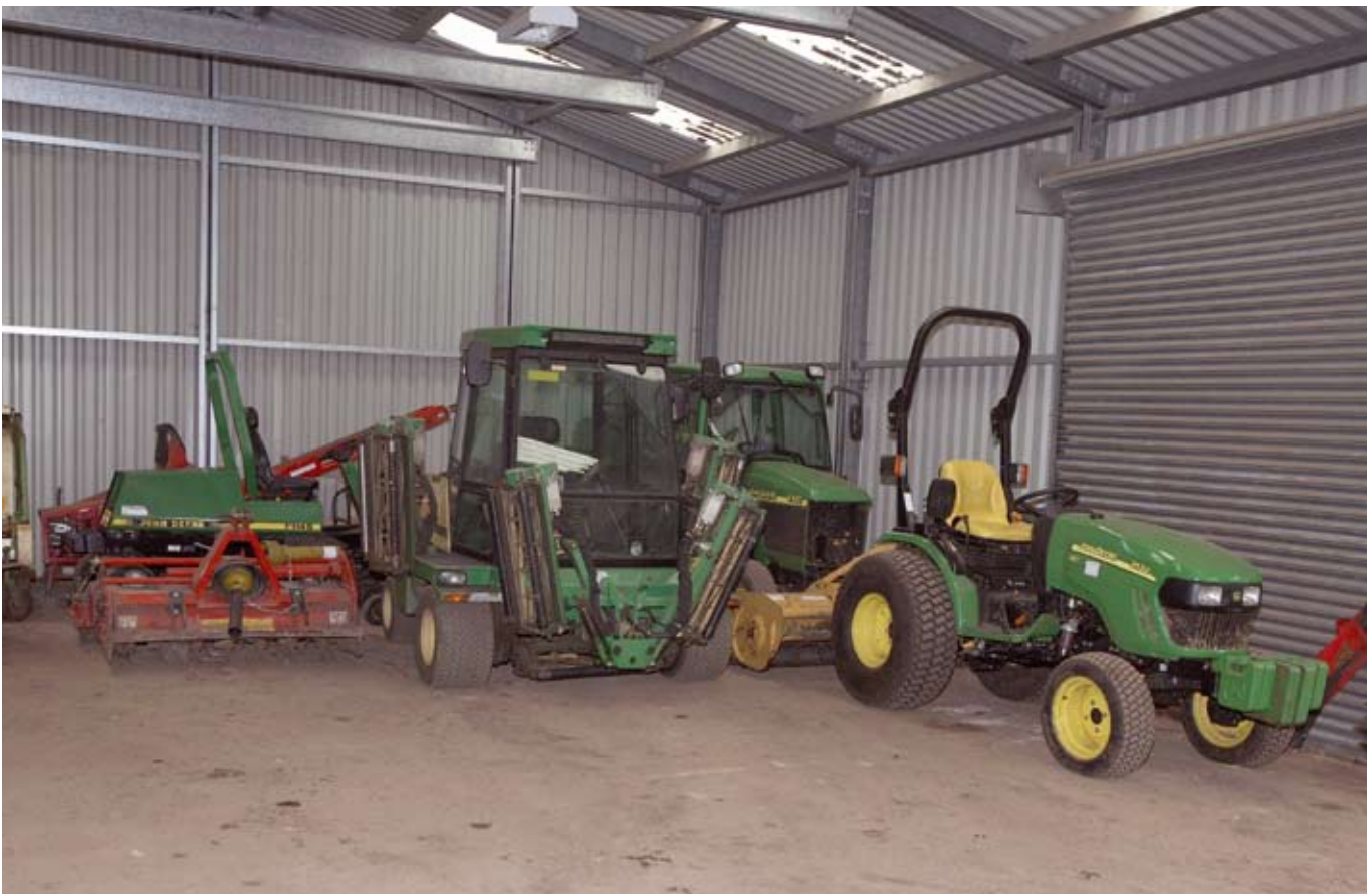
Storing equipment under cover, and keeping it clean, is a key maintenance task. If there is a shortage of workshop skills it can pay to hire in a trained mechanic to carry out routine and general servicing. Sharing resources with a neighbouring course can work well.
