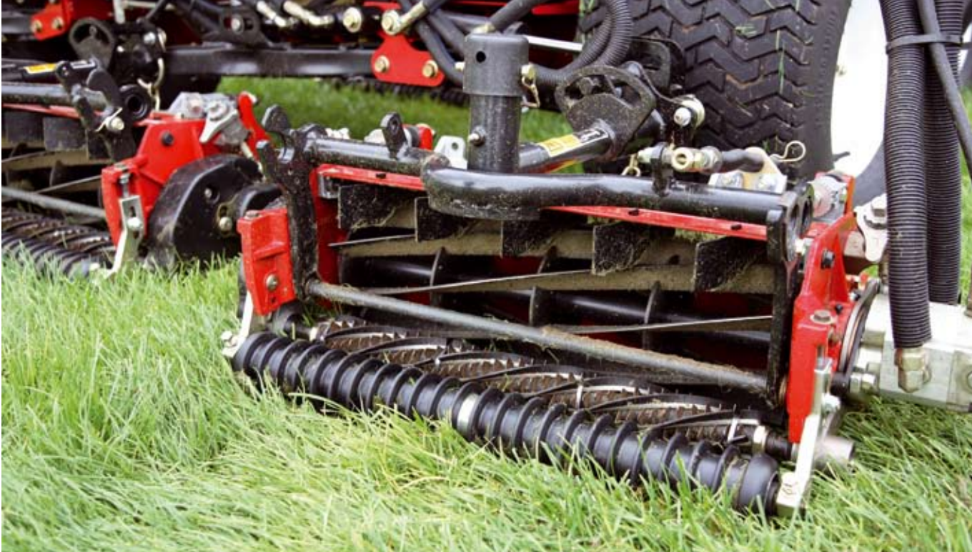
Modern units are easier to work on and remove for sharpening. Note also the access to the hydraulic drive motor and the routing of the hoses. Hydraulic leaks are increasingly rare on modern kit, but only if it has not been subject to unskilled maintenance attention.
