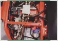
Make sure that battery leads are fitted tightly. Grease terminals and connectors to prevent corrosion. Check cells for electrolyte and top up where necessary
