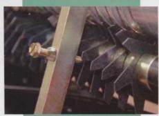
The setting bolt should just touch the groomer blade and then be taken back just a fraction to avoid contact
