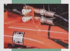
Check all of the hydraulic connectors for any sign of leakage
