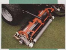
Turf groomers cut the lateral growth of the grass and stand the blades up to ensure a very consistent finish
