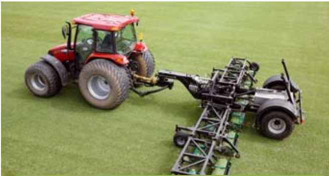
Turfmech's MaxiMow 13 and 17 trailed hydraulic gangs bring a new meaning to the term 'wide area mowing', with respective mowing widths of 9.06 and 11.75m. Innovative equipment, such as this, has helped specialist turf grass growers to contain costs and improve quality
