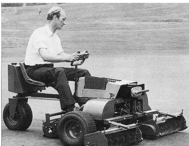
By the 1980s, Ransomes was producing its own greens mowers, the pictured Motor 180 and Tournament Triplex 171 being early examples. By 1984, the Triplex MarkII had a choice of brush or cutter attachments, quality of cut taking a useful step forwards
