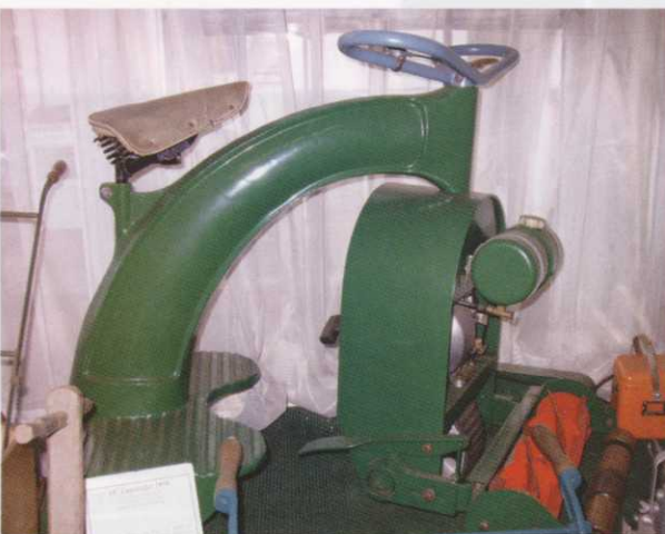
The Unique British Anzani, ride-on mower made of aluminium. It had one or two faults; one being if you went around a corner too fast, you'd tip and fall off!
