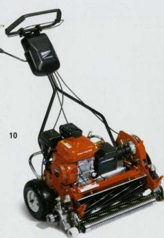
Although it is never possible to keep a mower in showroom condition, a good clean before putting it away is a key maintenance task. It pays to grease the machine as it is put away and then again when it is next used. Wipe off surplus lubricant.
