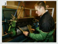
A small bend in a blade at the edge of the cylinder may be eased out using a light hammer. If in doubt, leave it to a specialist. With the mower up-ended, check for play in all bearings.
