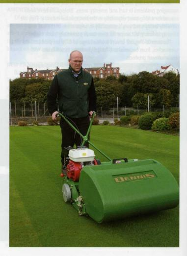
Moving on the cylinder, groomer, rollers and, where fitted, brushes, their setting is critical. Where applicable, the bottom knife to cylinder clearance 'air gap' needs to be maintained as recommended by the mower manufacturer. An air gap can reduce bottom knife wear by up to 50% and improves clippings flow for a smoother discharge. A quick check with a feeler gauge is all that is needed.
