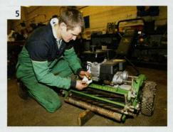
Checking the oil in a mower engine is a routine job, but remember the engine needs to be level to get a true reading. A block of wood under the front roller will do the trick. If the oil is dirty, change it. Look for leaks and clean off any spills before mowing.
