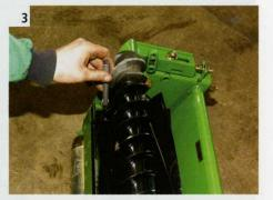
Where the cylinder and bottom knife operate with an air gap, check it is even across the face of the mower using a feeler gauge. Check with the manufacturer how this gap needs to be altered following back lapping. There are differences between makes and models.
