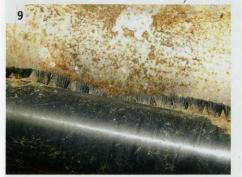
Set the roller power brush so the bristles lightly touch the roller. If the bristles are bent over they will typically not do their job and the power brush may need renewing. This setting needs periodic checking.
