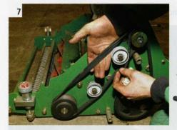
Belts need to be correctly tensioned to prevent slippage; an easy quarter of a turn on the belt is the typical maximum. If a belt drive machine is to be stored for an extended period, it can pay to remove the belts. If a belt shows signs of cracks or has been allowed to slip, it is best replaced.
