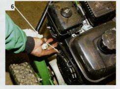
Ease out the starter cord, looking for damage particularly near the end. Any sign of fraying spells new cord time. It is easier to renew the cord than try to replace one that has snapped.
