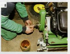
Transport wheels typically slide onto their shaft. To prevent them seizing, remove any corrosion with emery paper and apply a coat of copper grease. Check all fasteners, replacing any adjusters that are damaged or badly corroded.
