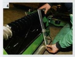
John Deere supplies its mowers with a simple setting bar that enables the rollers to be set so they run parallel to the bottom blade. This setting is critical on cylinder mowers.
