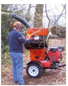
This powerful new model is equipped with 4 reversible heat treated steel chipper blades and a 76cm (30") diameter disc, driven by a 24hp Honda, which turns the disc at a remarkable 1500rpm via triple banded belt drive.
